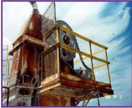
The sprocket and chain in this picture are not effectively guarded.
