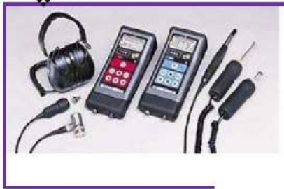
Equipment for testing bearings, Vibration and temperature.
